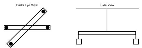
**Setup** - twisting the pendulum, releasing it, and measuring the period (change in direction to change in direction)
